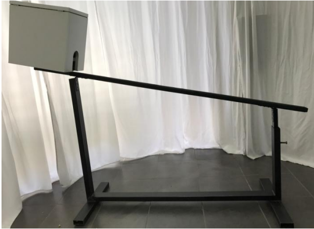
Figure 1. The apparatus for the evoked beam-walking test.
