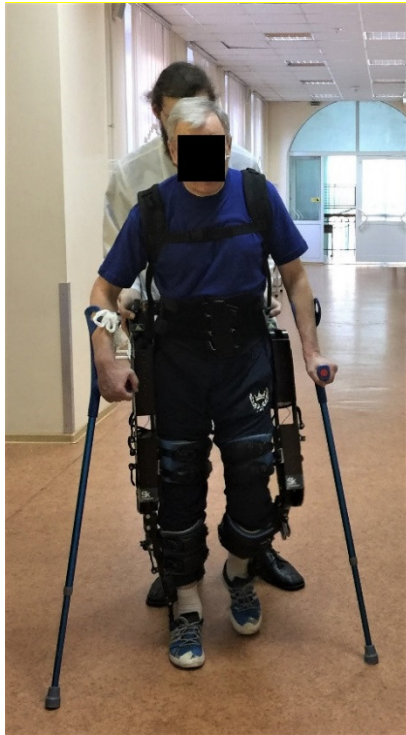
Figure 1. A patient walking with the ExoAtlet exoskeleton during the rehabilitation session.
