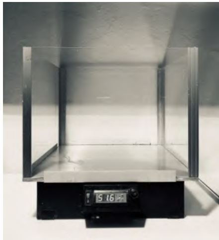
Figure 1. Apparatus used for the hot plate test.
